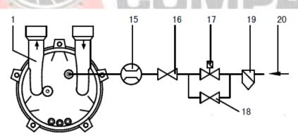
1. NCC vacuum pump 16. Control valve 15. Flow meter (optional)
