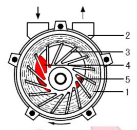
1 shows a sectional representation of the compression chamber, viewed from the perspective of the pump cover. An even surface is only required for its installation; there's no need for additional baseplates.
