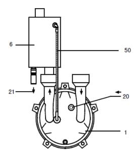
1. NCC pump 6. Liquid separator 20. Sealing liquid feed pipe 21. Working liquid discharge 50. Connection tube for cavitation protection
