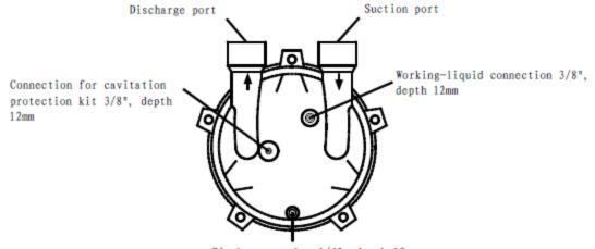
Discharge outlet 1/4", depth 12mm
