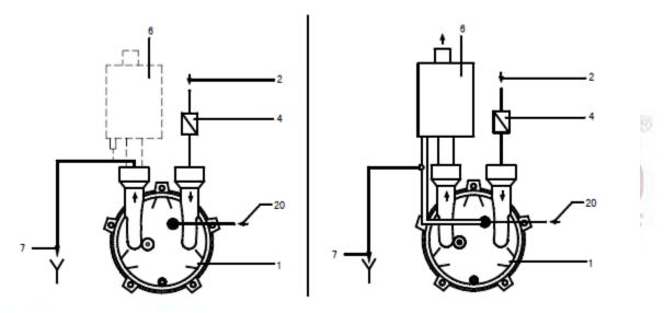
1. NCC pump 2. Suction pipe 4. Non-return valve 6. Liquid separator 7. Overflow 20. Sealing liquid feed pipe **Fig. 6 Different ways of supplying sealing liquid**
