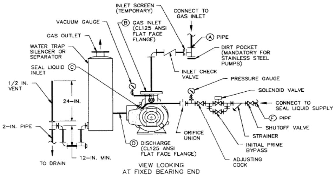
Fig. 2.1b Typical Vacuum pump piping connections for NC-6 & NC-7
