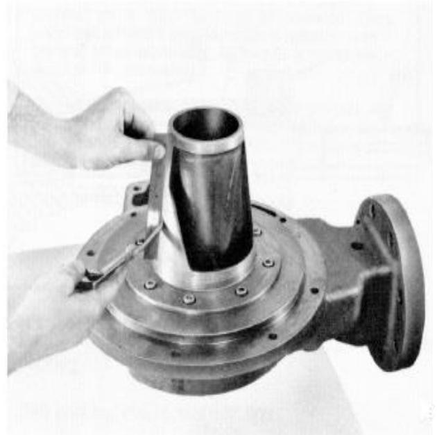
Fig. 5.4 Checking cone for wear
