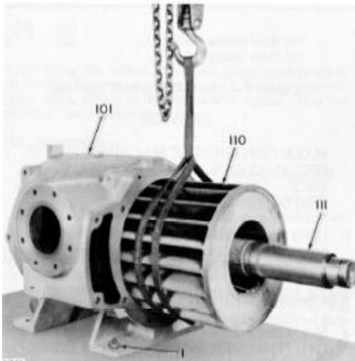
Fig. 5.6b Installing Rotor and Shaft Assembly for NC-6 & NC-7
