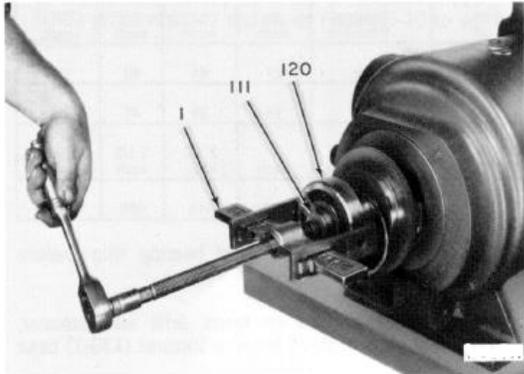
1. Bearing Puller      2. Shaft      3. Fixed Bearing
