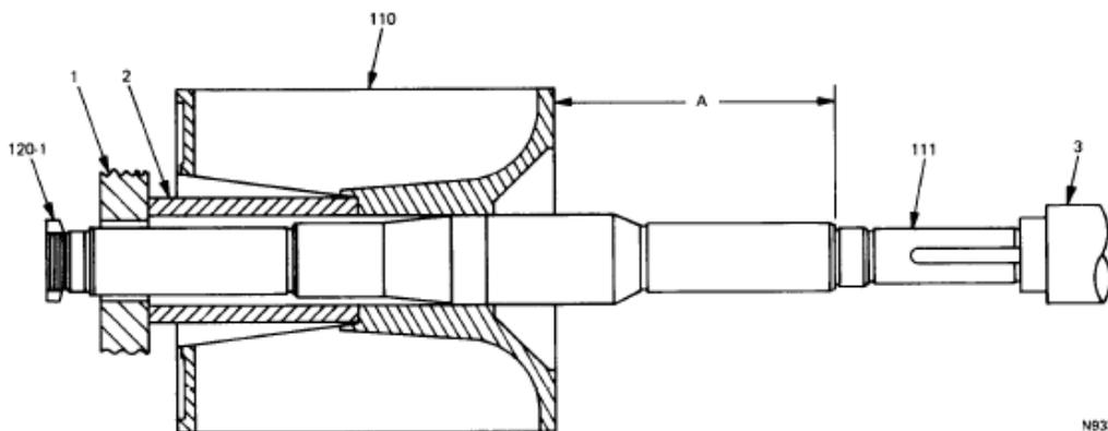
Fig. 5.5b Pressing Rotor Onto Shaft for NC-6 & NC-7
