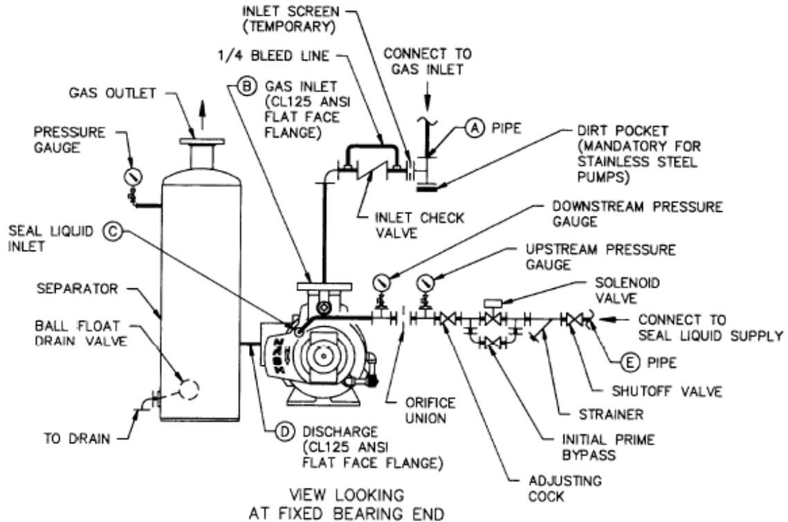
Fig. 2.2b Typical Compressor Piping Connections for NC-6 & NC-7
