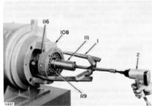
1. Bearing Puller      108. Floating Bearing Bracket      116. Floating Bearing Inner Cap
