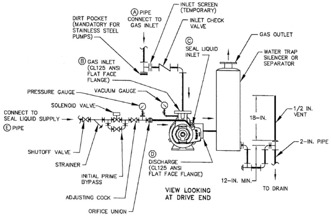
Fig. 2.1a Typical Vacuum pump piping connections for NC2 to NC-5
