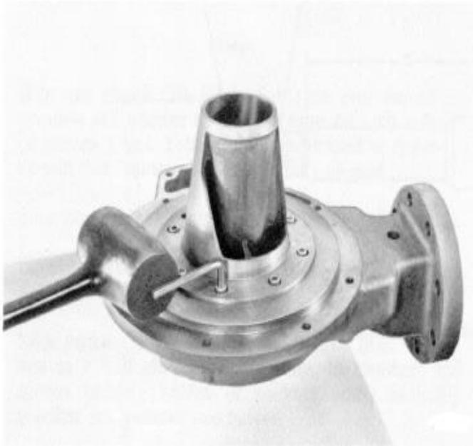
Fig. 5.3 Loosening Cone Screws
