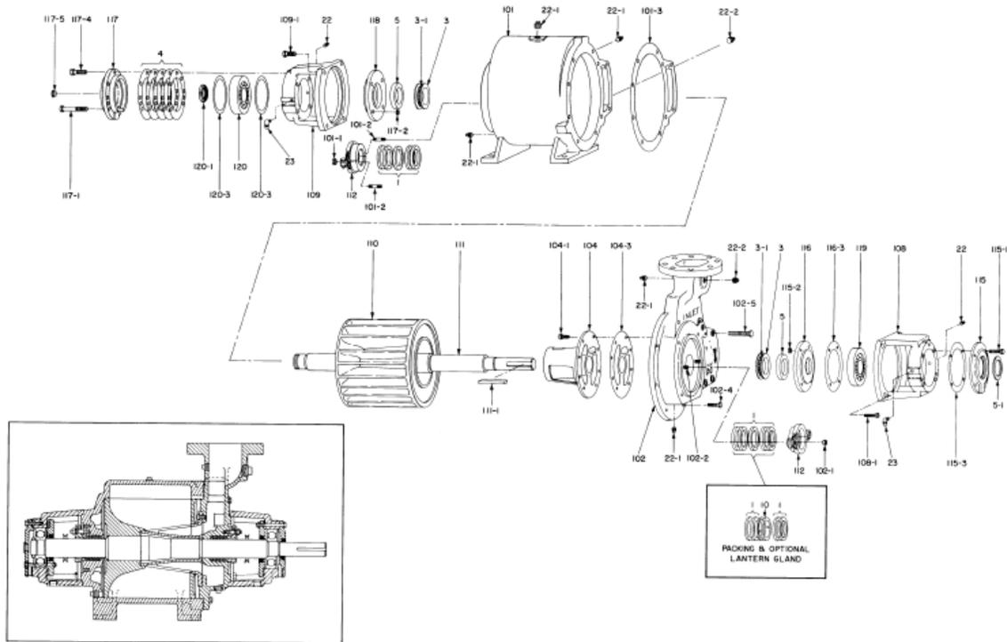
Fig. 5.12 NES exploded view NC-2, NC-3, NC-4, and NC-5 pumps and compressor
