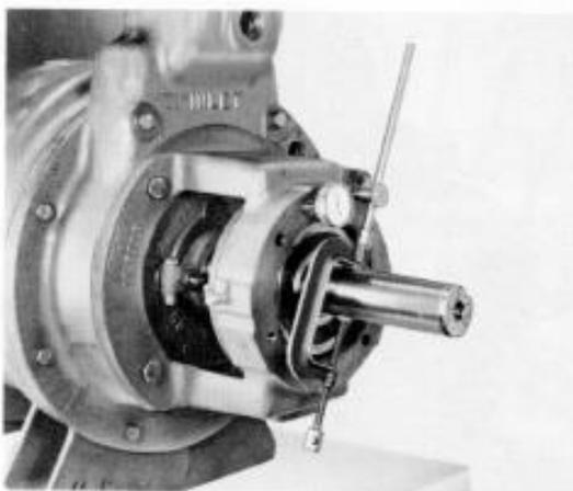
Fig. 5.9 Measuring End Travel at Floating Bearing End
