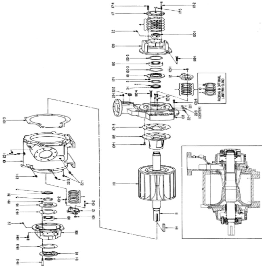
Fig. 5.13 NES exploded view NC-6band NC-7 pumps and compressor
