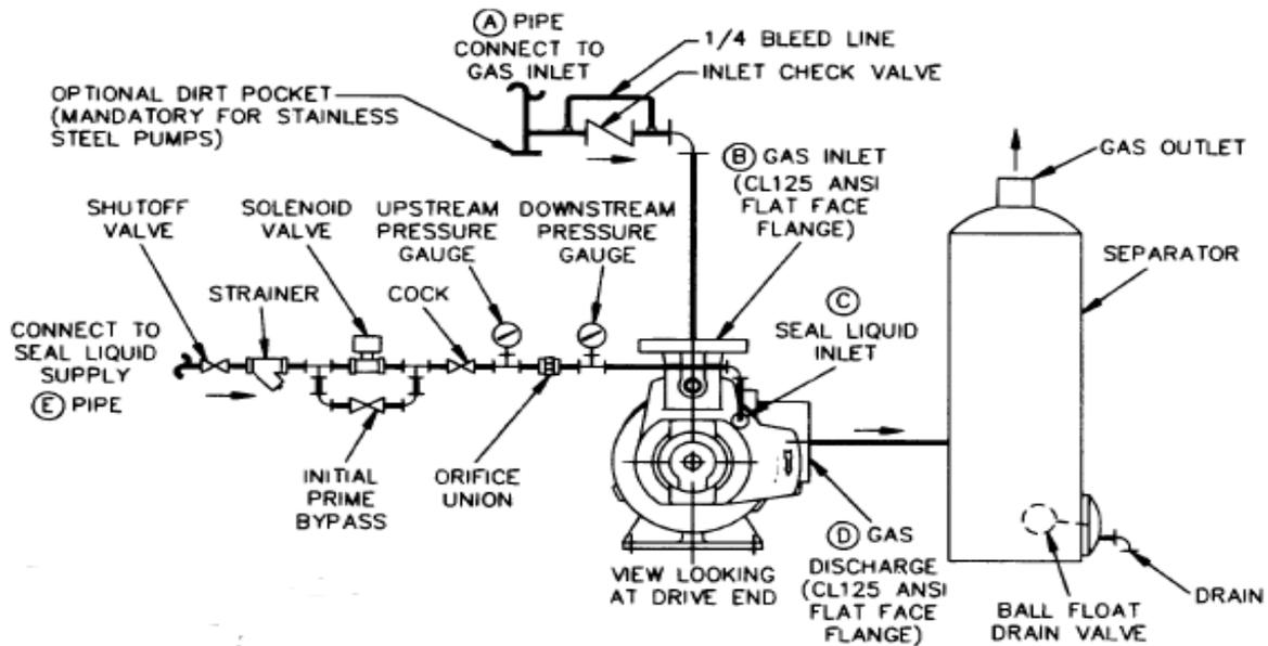
Fig. 2.2a Typical Compressor Piping Connections for NC-2 to NC-5
