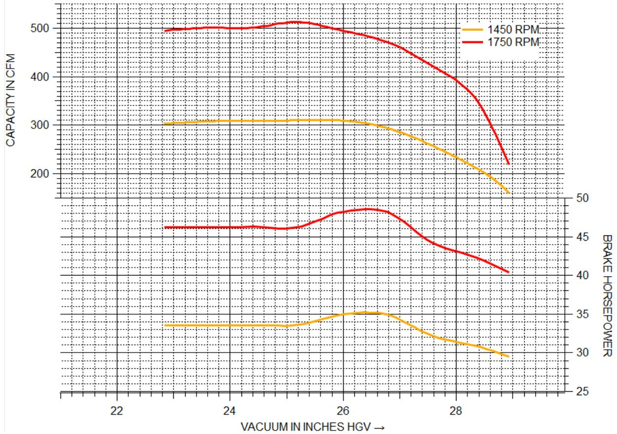
\*The dry air curves above apply to cast iron, direct-driven equipment. Stainless steel equipment may experience  $\pm 10\%$  performance due to stringent manufacturing specifications.
