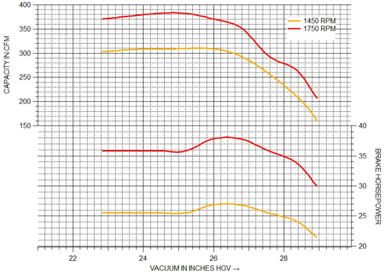
\*The dry air curves above apply to cast iron, direct-driven equipment. Stainless steel equipment may experience  $\pm 10\%$  performance due to stringent manufacturing specifications on dimensional tolerancing.
