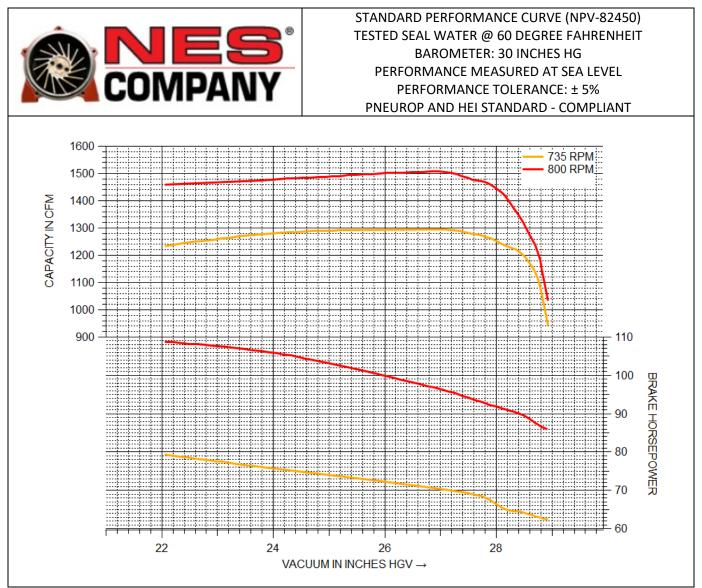
\*The dry air curves above apply to cast iron, direct-driven equipment. Stainless steel equipment may experience ± 10% performance due to stringent manufacturing specifications.
