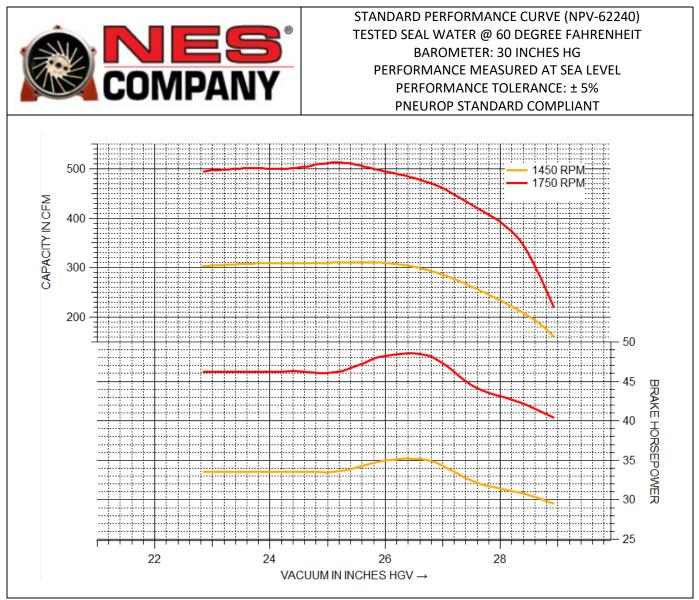
\*The dry air curves above apply to cast iron, direct-driven equipment. Stainless steel equipment may experience ± 10% performance due to stringent manufacturing specifications.
