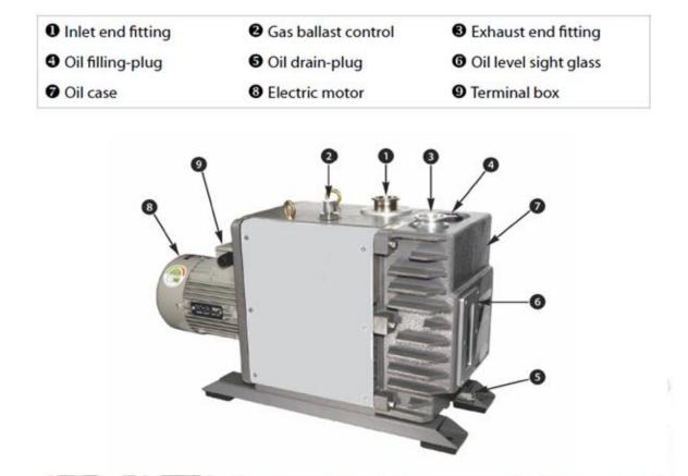
Fig. 4 A typical NTRV100/NTRV180 high vacuum rotary vane pump
