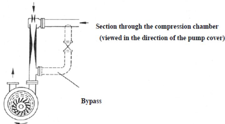
**Fig. 8 Operation with gas ejector**
