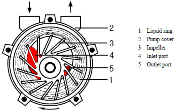
Fig. 1 Sectional view through the compression chamber
