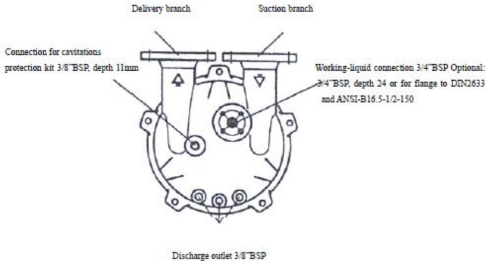
**Fig. 4 Pipe Connection of NCC 115-350 stainless steel version**
