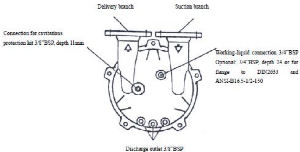
**Fig. 3 Pipe Connection of NCC 115-350 cast iron version**
