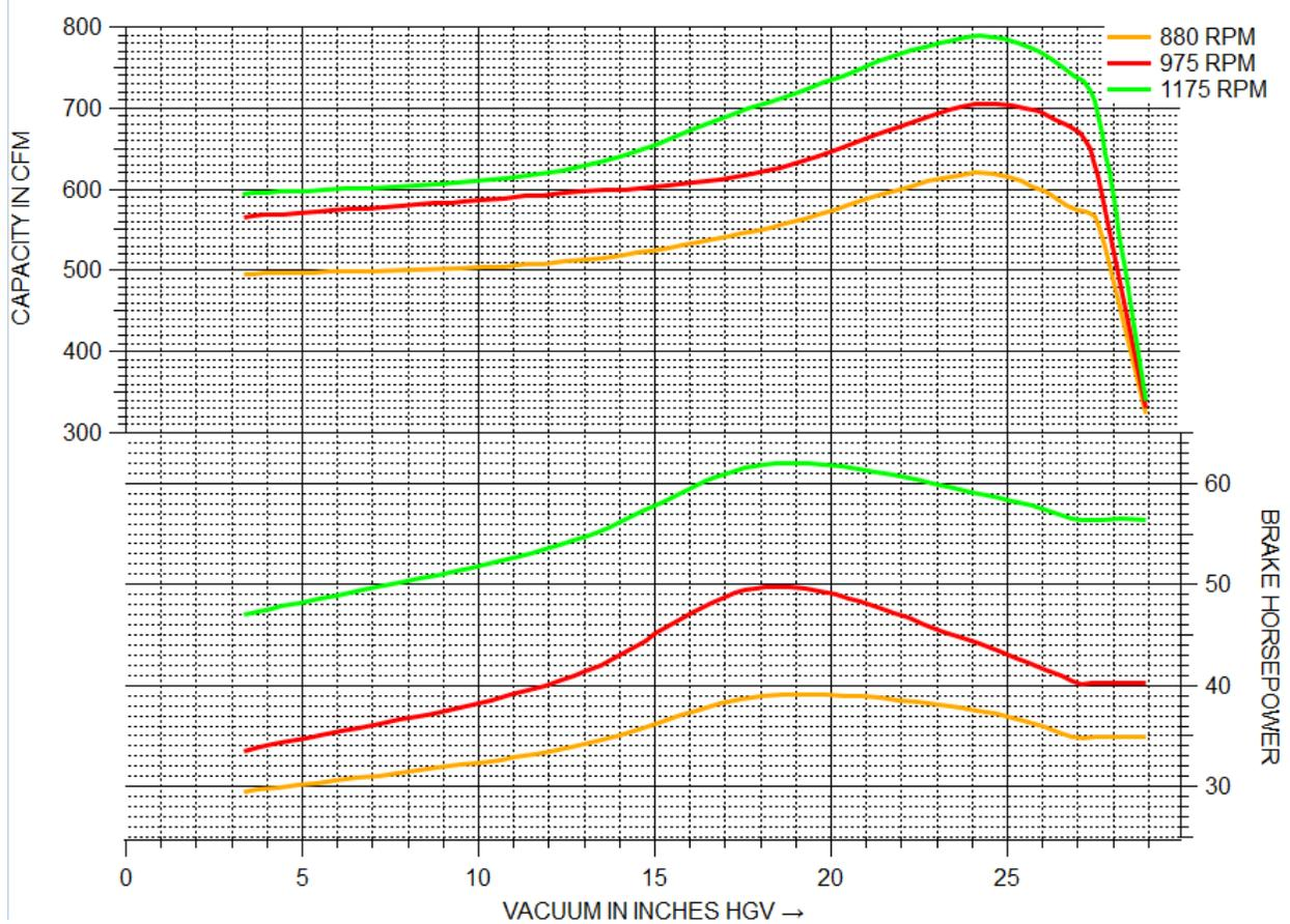
\*The dry air curves above apply to cast iron, direct-driven equipment. Stainless steel equipment may experience ± 10% performance due to stringent manufacturing specifications.
